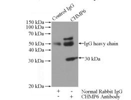
IP Result of anti-CHMP6 (IP:Catalog No:109236, 4ug; Detection:Catalog No:109236 1:500) with mouse testis tissue lysate 2400ug.
