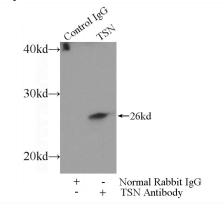
IP Result of anti-TSN (IP:Catalog No:116436, 3ug; Detection:Catalog No:116436 1:300) with MCF-7 cells lysate 1600ug.
