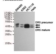
Western blot detection of DR5 in SW480,K562,HCT116 and Hela cell lysates using DR5 mouse mAb (1:1000 diluted).Predicted band size:40/48KDa.Observed band size:40/48KDa.
