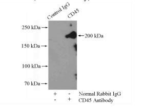
IP Result of anti-CD45 (IP:Catalog No:109125, 4ug; Detection:Catalog No:109125 1:300) with mouse spleen tissue lysate 4800ug.
