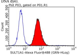
1X10^6 HepG2 cells were stained with 0.2ug SULT1A1 antibody (Catalog No:115825, red) and control antibody (blue). Fixed with 90% MeOH blocked with 3% BSA (30 min). Alexa Fluor 488-congugated AffiniPure Goat Anti-Rabbit IgG(H+L) with dilution 1:1000.
