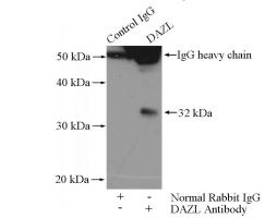
IP Result of anti-DAZL (IP:Catalog No:109874, 4ug; Detection:Catalog No:109874 1:500) with mouse testis tissue lysate 4400ug.
