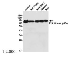
Western blot detection of PI3 Kinase  $p85\alpha$  in Jurkat,Rat Brain,Raw264.7,Ramos,Raji cell lysates using PI3 Kinase  $p85\alpha$  (1C8) Mouse mAb(1:1000 diluted).Predicted band size:85KDa.Observed band size:85KDa.
