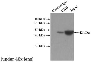
IP Result of anti-CKB (IP:Catalog No:109543, 4ug; Detection:Catalog No:109543 1:500) with mouse brain tissue lysate 4000ug.
