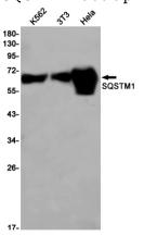
Western blot detection of SQSTM1 in K562,3T3,Hela cell lysates using SQSTM1 Rabbit pAb(1:1000 diluted).Predicted band size:48kDa.Observed band size:62kDa.
