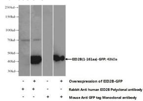
Transfected HEK-293 cells were subjected to SDS PAGE followed by western blot with Catalog No:110171(EID2B Antibody) at dilution of 1:1000
