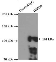
IP Result of anti-DDX58 (IP:Catalog No:109841, 4ug; Detection:Catalog No:109841 1:600) with A431 cells lysate 1200ug.
