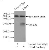
IP Result of anti-HBA1 (IP:Catalog No:111287, 4ug; Detection:Catalog No:111287 1:500) with mouse liver tissue lysate 4000ug.
