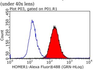
1X10^6 HeLa cells were stained with 0.2ug HOMER1 antibody (Catalog No:111517, red) and control antibody (blue). Fixed with 90% MeOH blocked with 3% BSA (30 min). Alexa Fluor 488-congugated AffiniPure Goat Anti-Rabbit IgG(H+L) with dilution 1:1000.
