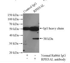
IP Result of anti-Noc2 (IP:Catalog No:114807, 4ug; Detection:Catalog No:114807 1:500) with HepG2 cells lysate 2400ug.
