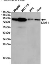
Western blot analysis of extracts from HepG2, HCT116, 3T3 and Hela cells using Stat1 Rabbit pAb at 1:1000 dilution. Predicted band size: 84kDa. Observed band size: 84kDa.
